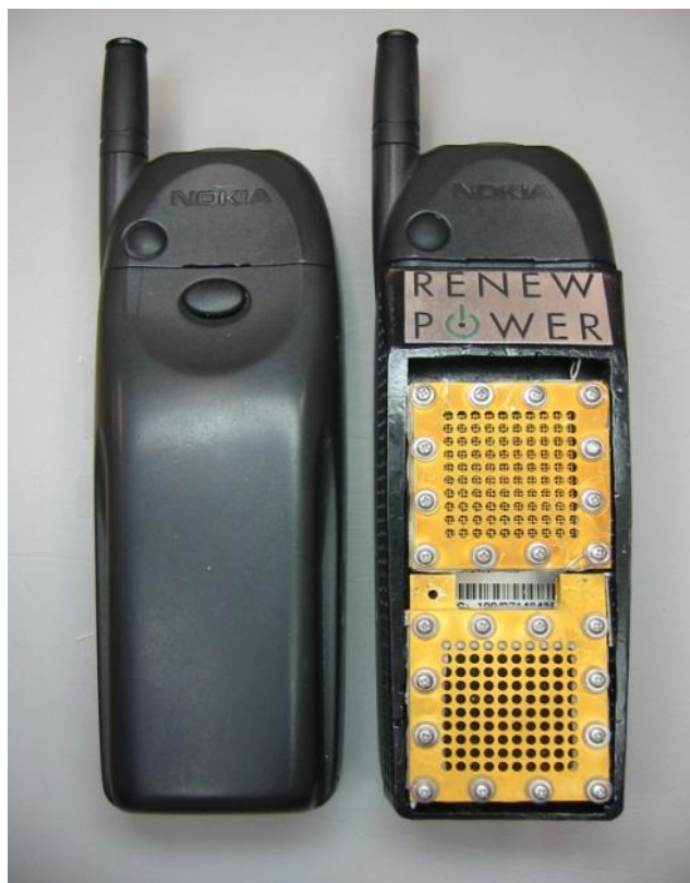
Figure 4.1. A formic acid fuel cell demonstrated as a power source for a wireless phone.
