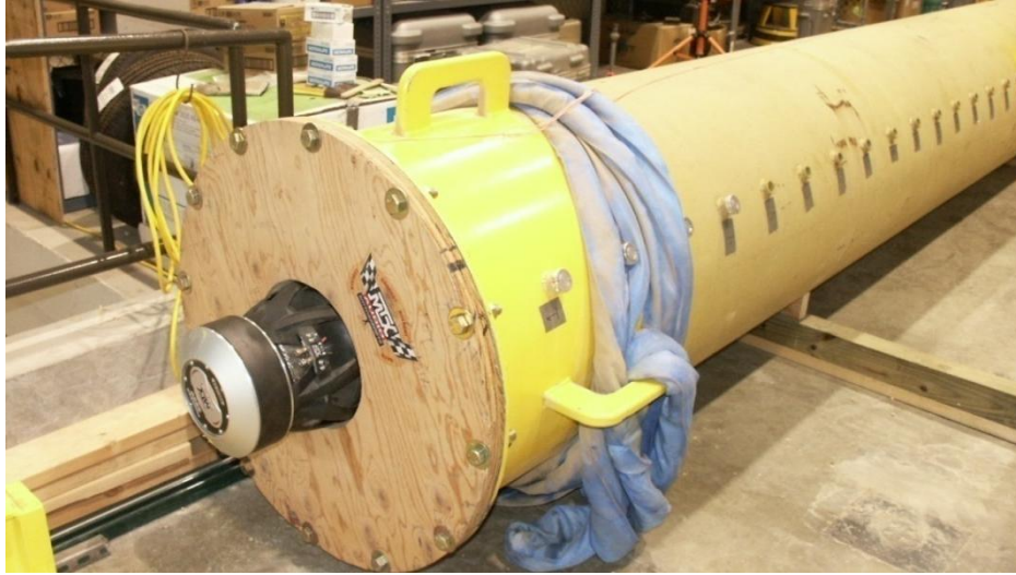
Figure 3.2: 12 in speaker set in the top of the impedance tube. Courtesy of Tim Eggerding.
