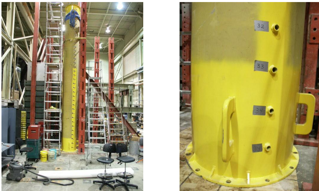
Figure 3.1: CERL impedance tube (left) with close-up of microphone ports (right).
