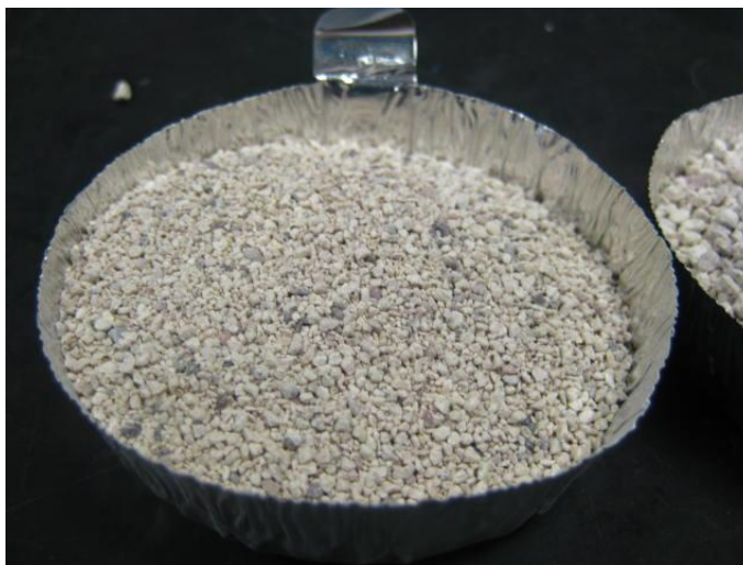
Figure 2.6. Photograph of clinoptilolite from St. Cloud Mines, mesh size 14x40.
