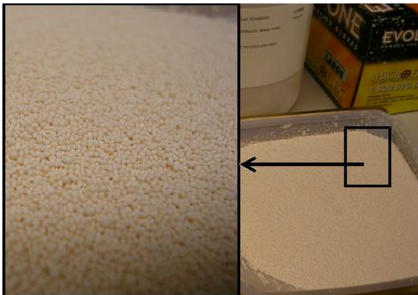
Figure 3.1. Photographs of Amberlite® IRA-92 anion exchange resin.
