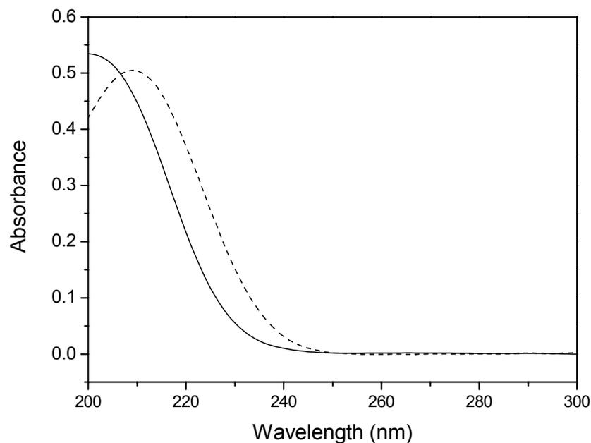
**Figure 8.** Absorption spectrum of 0.08 mM nitrite (solid) and 0.08 mM nitrate (dash). Nitrate peak occurs at 210 nm and no band appears at 300 nm at such dilute concentrations.
