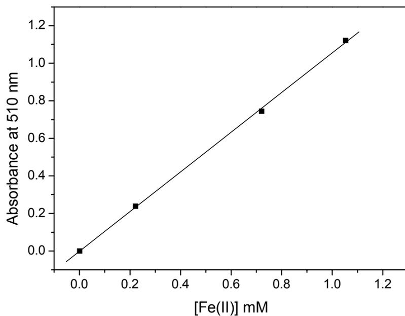
**Figure 9.** Sample calibration curve for Fe(II) analysis.  $R^2 = 0.99974$ .
