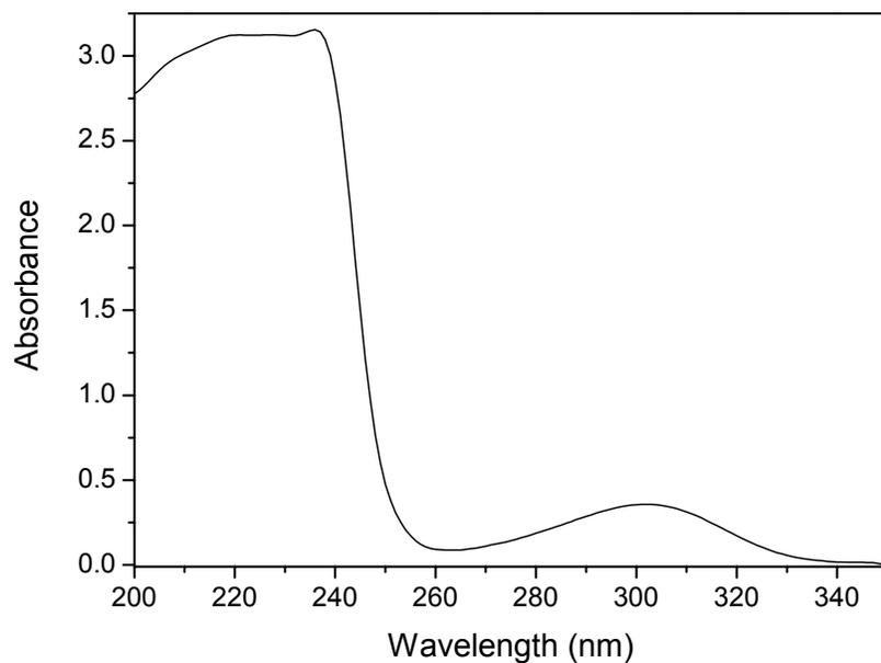
**Figure 6.** Absorption spectrum of 0.50 mM nitrate. Band at 300 nm is usable in this concentration range. The 200 nm band is stretched and absorbance values are much greater than 1.0.
