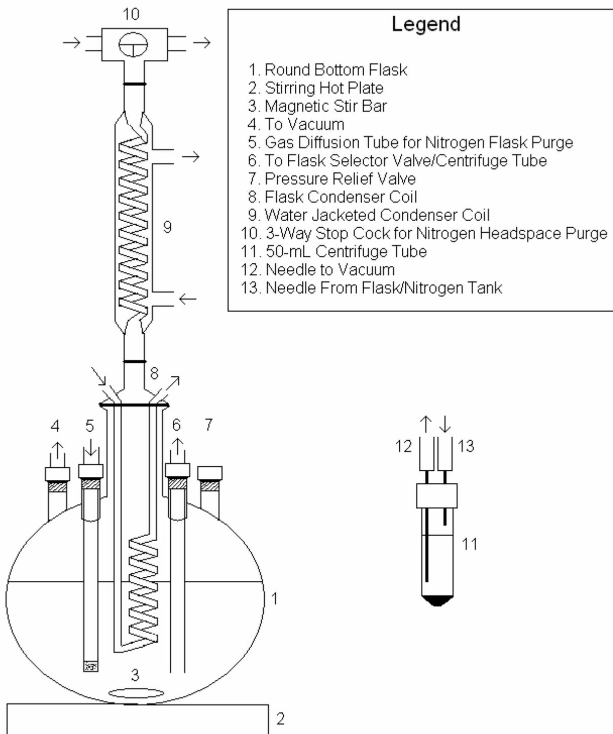
**Figure 5.** Diagram of washing apparatus
