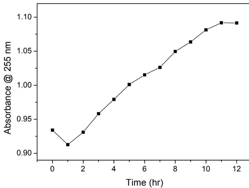
**Figure 25.** Separated ferric-oxygen charge transfer values for oxygenated zero-valent iron and clay flow reactor experiment.
