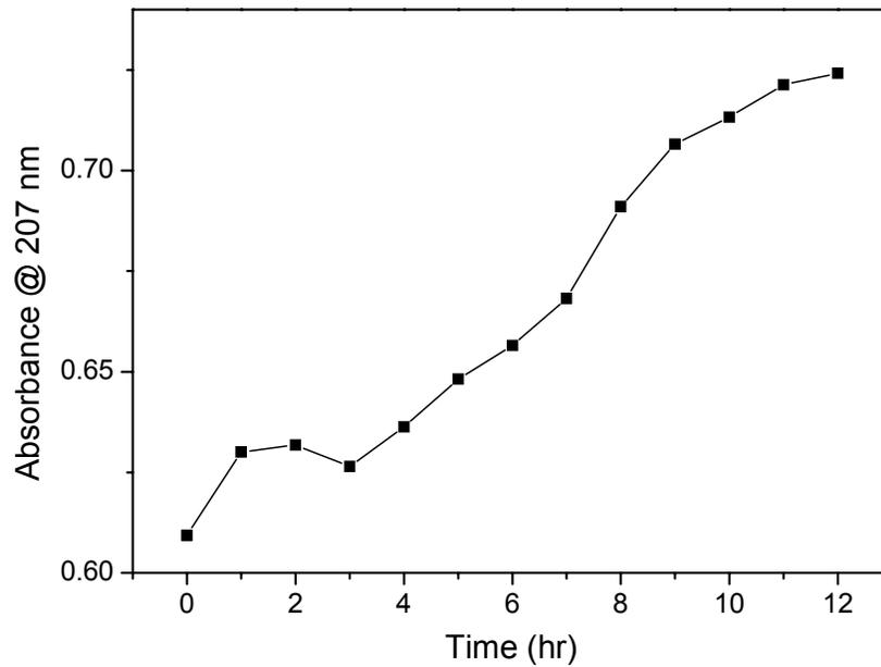
**Figure 24.** Separated nitrate peak values for oxygenated zero-valent iron and clay flow reactor experiment.
