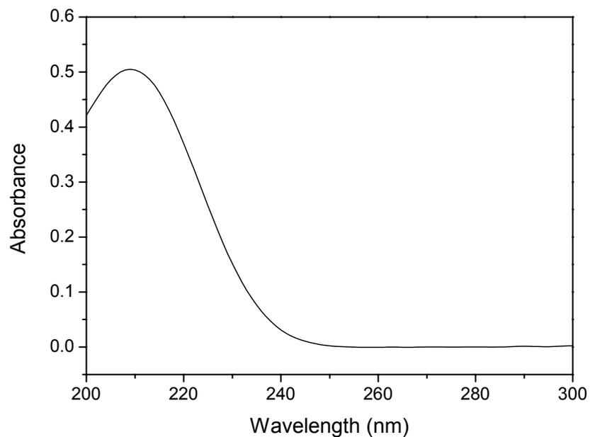
**Figure 7.** Absorption spectrum of 0.08 mM nitrite. Peak maximum is at 210 nm.
