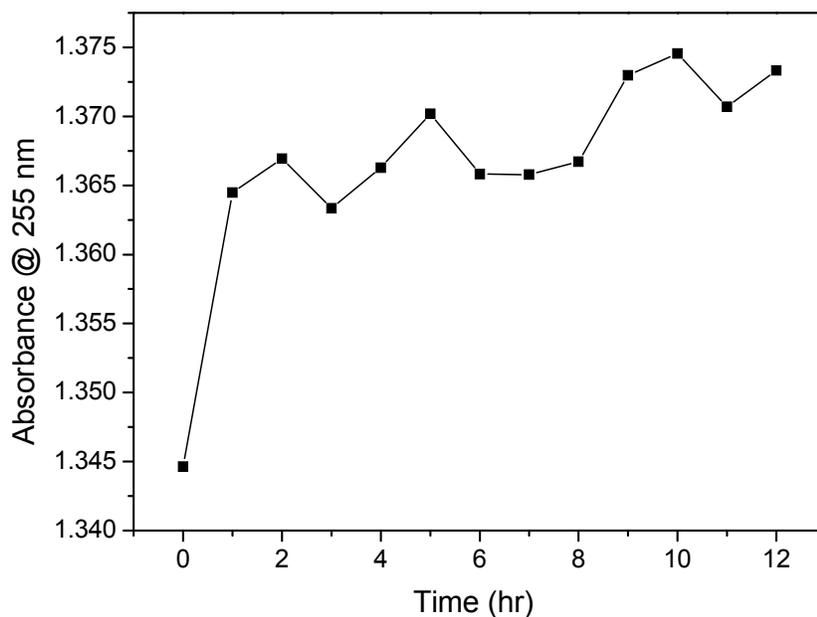
**Figure 23.** Separated ferric-oxygen charge transfer values for deoxygenated zero-valent iron and clay flow reactor experiment.
