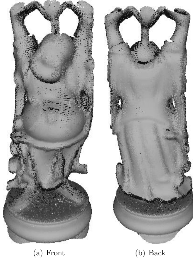
Figure 7.4: Visualization of the set of points registered using SDR with noise-free synthetic points and estimated normals.
