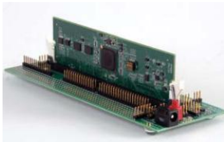
Figure 9: The F28335 controlCard [13]
