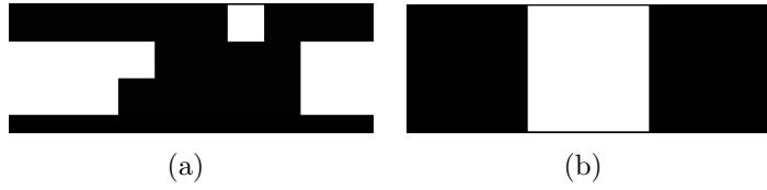
Figure 2.7: Masked lateral image (a) original image and (b) binary texture classification mask for image, where black is “non-ballast” and white is “ballast.”
