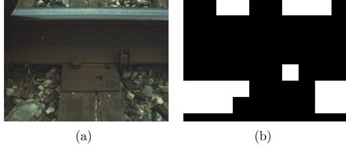
Figure 2.7: Masked lateral image (a) original image and (b) binary texture classification mask for image, where black is “non-ballast” and white is “ballast.”
