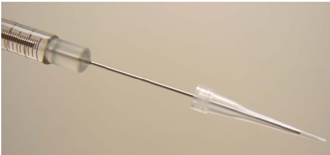
Figure 3.2 Image of elution method after peptide collection and desalting on a C18-packed pipette (ZipTip). Shown is a 0.6 \mu\text{L} ZipTip to be eluted with 70% ACN into 5-6 0.2 \mu\text{L} spots through the use of slow manual control of a 100 \mu\text{L} blunt tip syringe directly onto a MALDI target.
