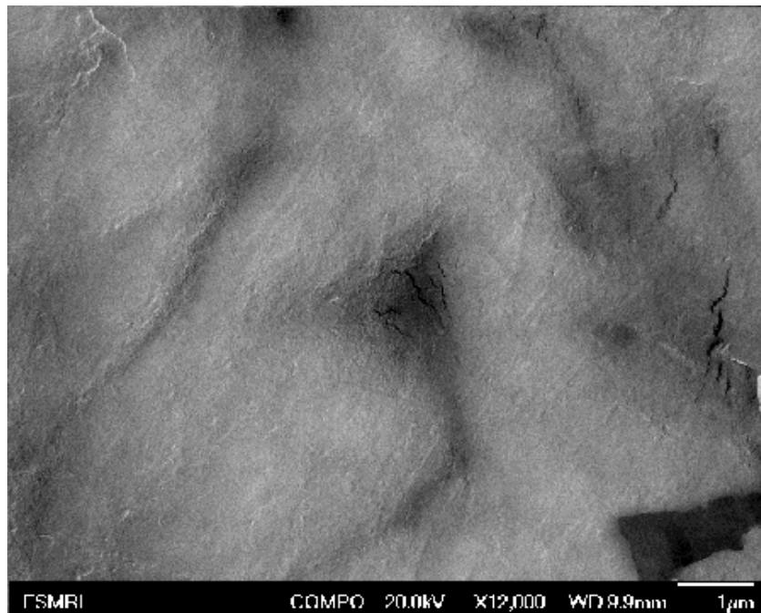
Figure 12 SEM Backscatter image of one indent on 30 month sample (12,000 zoom).
