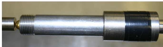
Figure 2.10. Image of the one dimensional sphere holder with one end cap in place.
