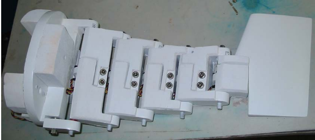
Figure 3.7 – Robot fish tail, fully assembled
