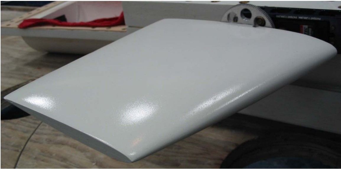
Figure 3.9 – Robot pectoral fin control surface
