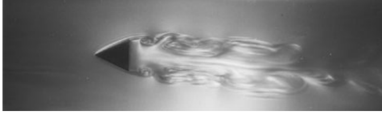
Figure 2.1 – Visualization of Kalliroscope fluid flow field in vicinity of triangle cross section (photograph courtesy of Kalliroscope.com, 2012)]
