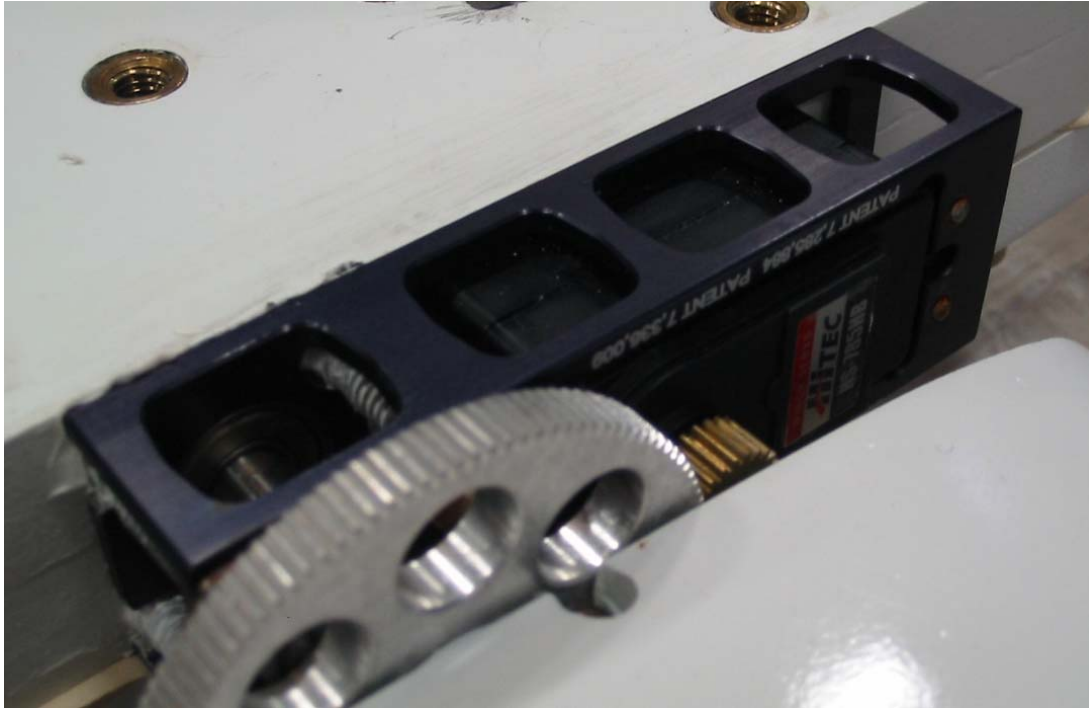
Figure 3.10 – Robot pectoral fin control surface actuator
