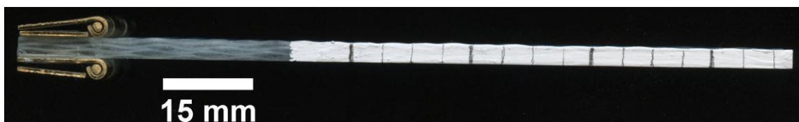
Figure 2.4. A plain double cantilever beam specimen with 5 mm demarcations. Darker marks indicate 20 mm segments.
