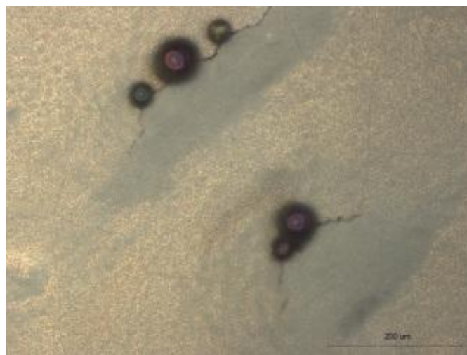
Figure 32 Indium release layer bubbling up through YSZ after sintering
