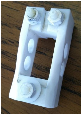
Figure 13 Teflon sample holder for EPD
