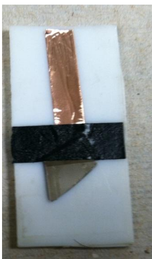
Figure 14 Sample mounted to Teflon backing plate with carbon tape. Copper tape is used to ensure sample is negatively charged.
