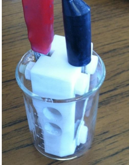
Figure 15 Teflon deposition cell with alligator clips attached to anode (SS plate) and cathode (Teflon plate with sample mounted to it)
