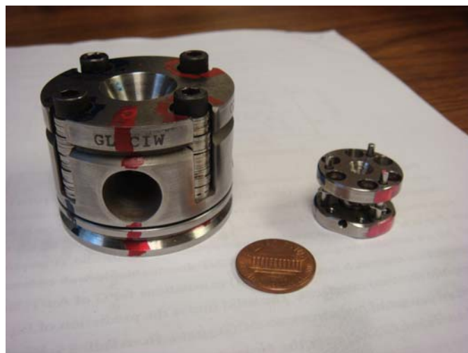
Fig. 2.7. Two types of the opposing-plate diamond and SiC anvil cells used in this thesis work. A penny is included as the scale bar of anvil cells.
