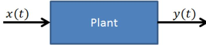
Figure 3.4: Basic example of an open-loop system.
