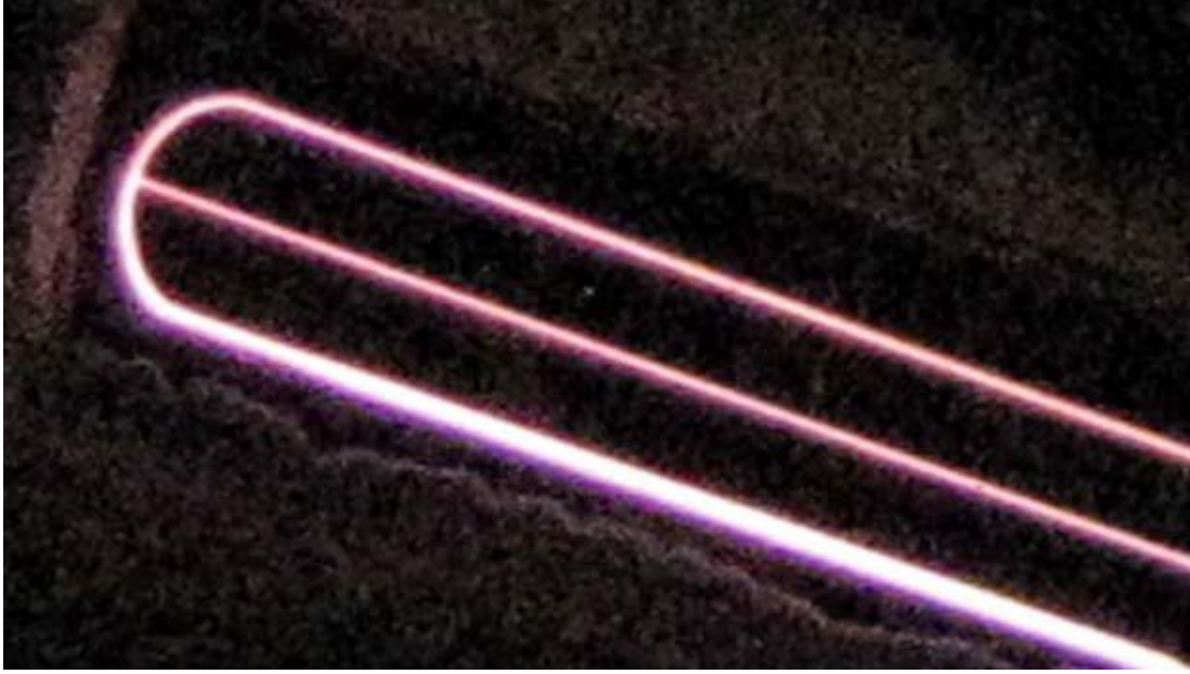
Figure 2.3: Undesired surface discharge on the electrode edge [9].
