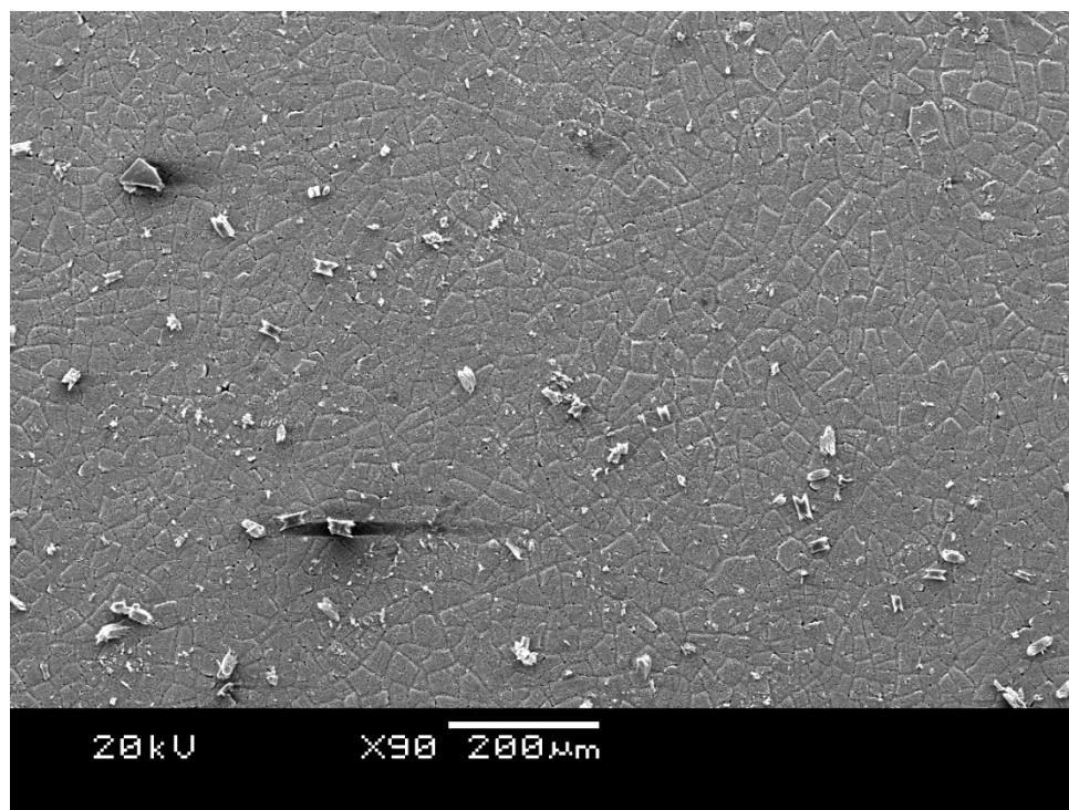
Figure 19. Scanning electron micrograph of TiO 2 film following 4 d of exposure to GW matrix when treating micropollutants, then 1 d of rinsing with oxalic acid.
