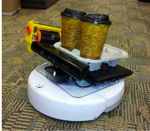
Figure 2.1: Our robot, Clarke, includes an iRobot Create, a netbook, and a Kinect.
