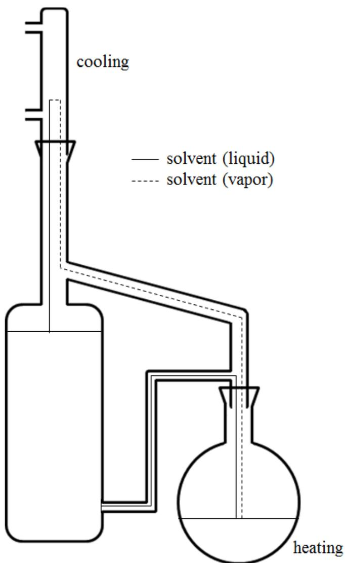
Aroma extracts were obtained by continuous liquid-liquid extraction (LLCE, Figure 3.1). A continuous extraction apparatus (#Z562440; Sigma Aldrich, St Louis, MO) was attached to both a 7-inch-long condenser and a 300 mL receiving flask. The condenser was cooled to a temperature of 4° C, while the flask was heated to a temperature appropriate for steady evaporation of solvent. To the system were added 150 mL of dichloromethane as the solvent, 100 mL of rum, and 425 mL of deodorized water.
