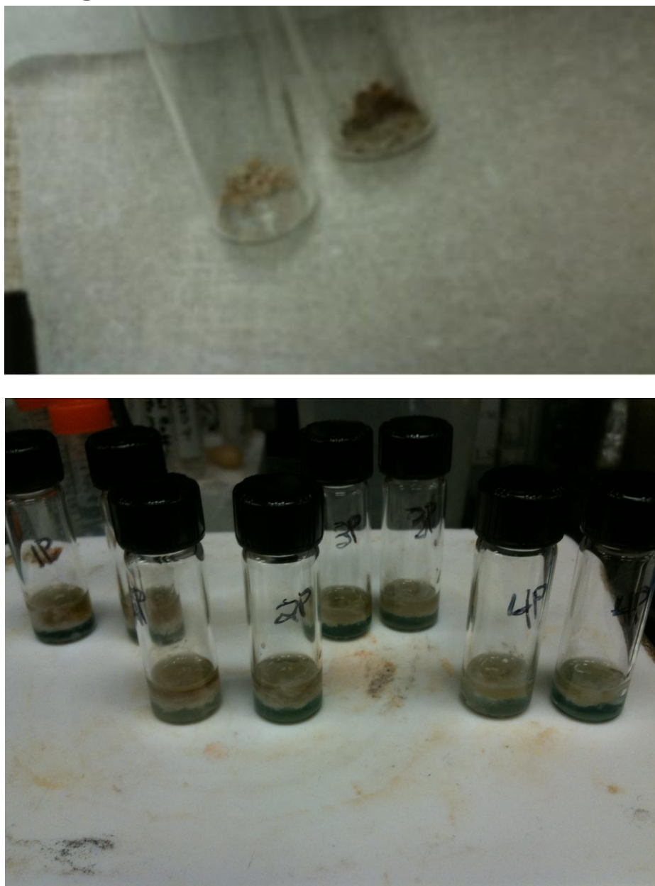
Figure 11. Physical appearance of two different 5-mutant Azurin-generated polymers. On Top: Styrene only (left) and Styrene+Iridium Chloride (50 equivalents, right). On Bottom: Pyrrole polymerization, showing the rapid clouding and thickening that takes place immediately after pyrrole is added, even without mixing. Conditions: 0.5 mL pyrrole is added to 0.5 mL 250 \mu M 5-mutant Azurin. A cloudy, dark, gooey layer has formed within 5 minutes of addition in the top (pyrrole) layer. With additional time, this layer will turn to black.
