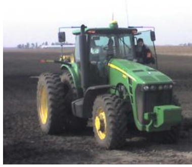
Figure 5.1 John Deere 8330 tractor equipped with StarFire TM RTK receiver and an integrated AutoTrac TM steering system
