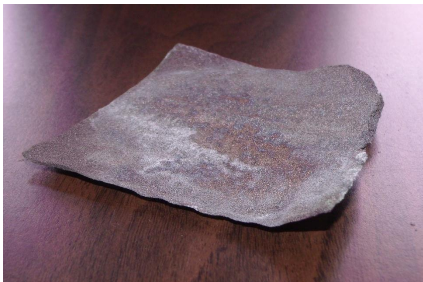
Figure 18: Nickel Foam Degradation
