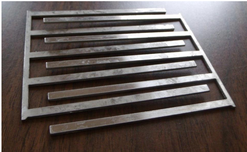
Figure 12: Deformed Stainless Steel Channels
