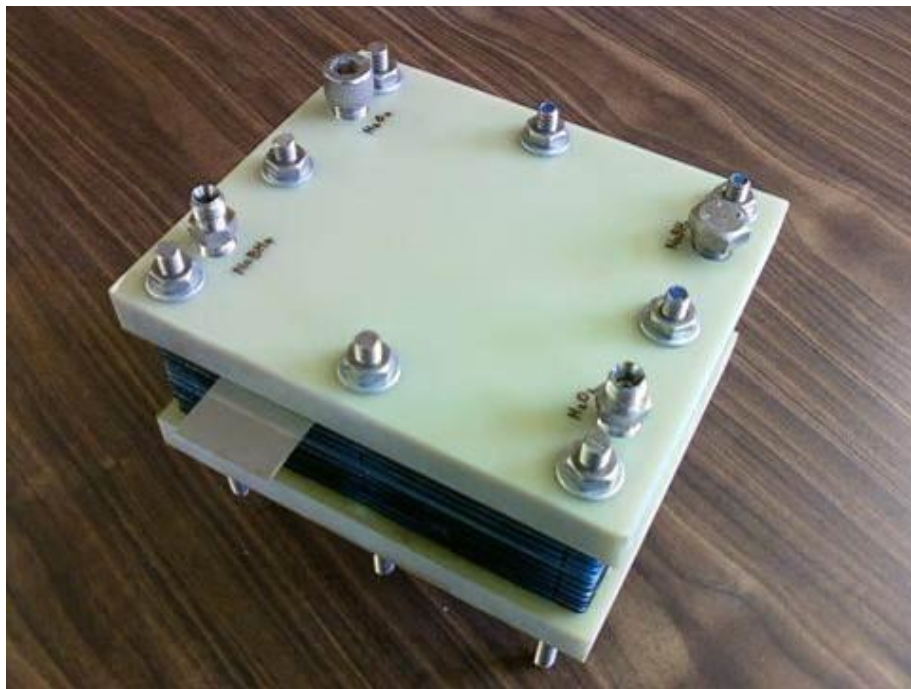
Figure 7: Fully Assembled Stack
