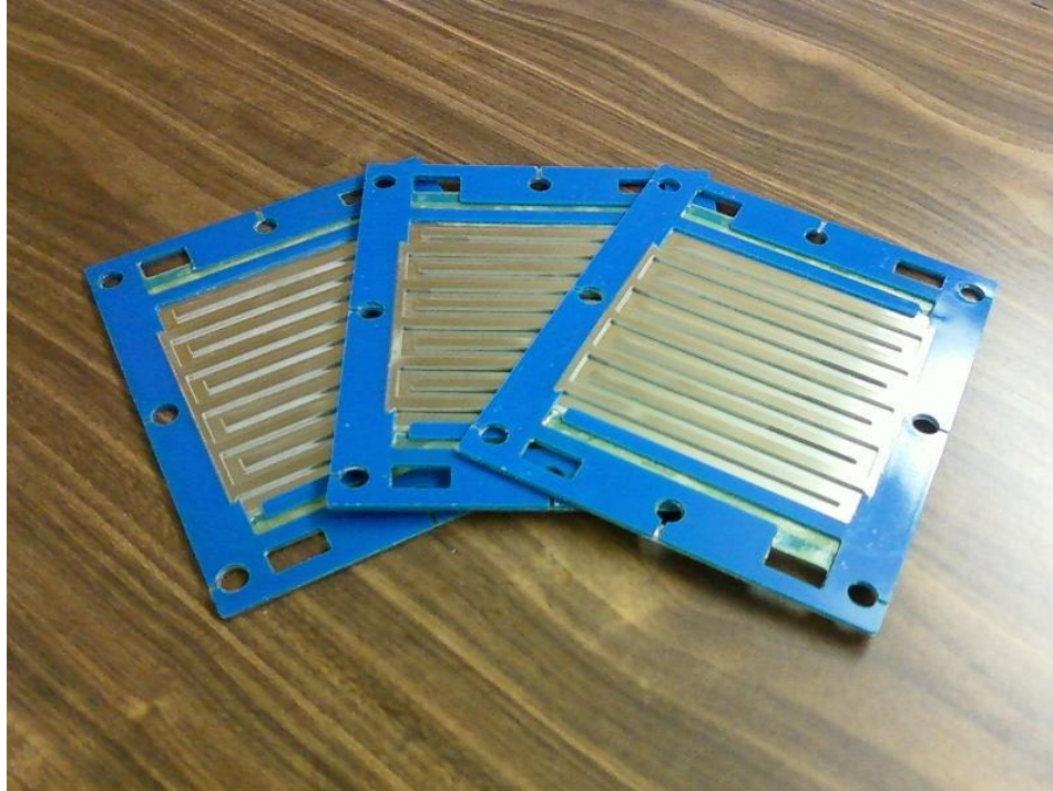
Figure 4: Manufactured Bipolar Plates [21]
