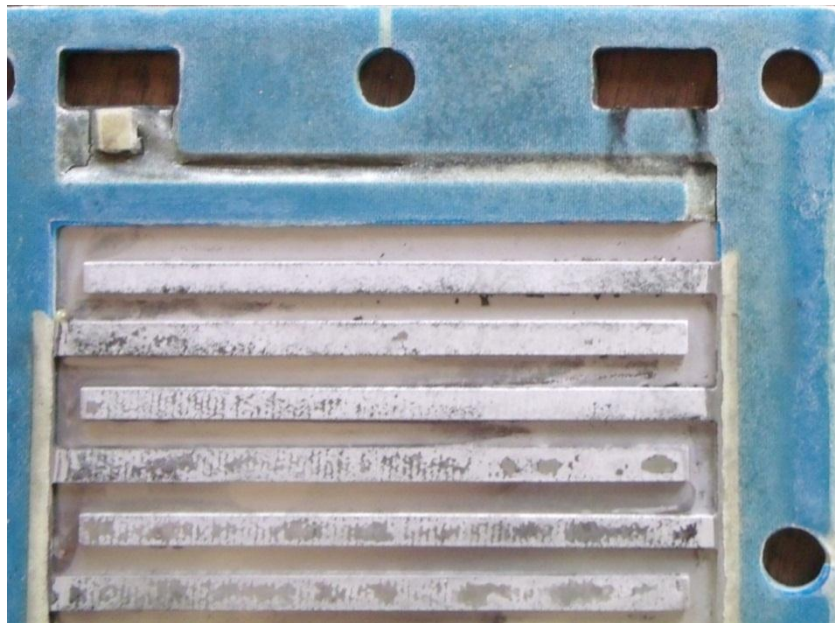
Figure 10: Flow Marks on Side 1
