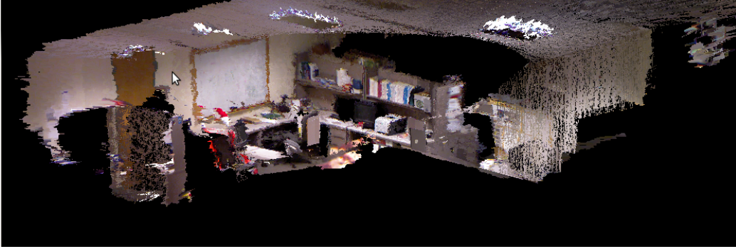
Figure 3.2: A map generated by the RGB-D SLAM System.
