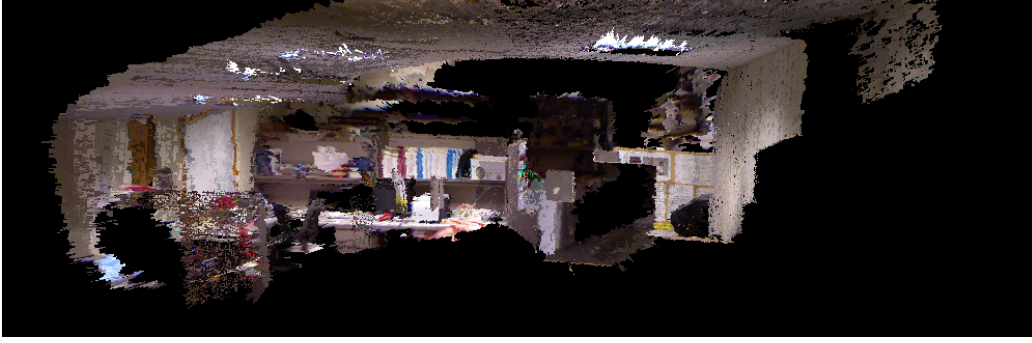
Figure 6.2: A map generated by the RGB-D SLAM System.
