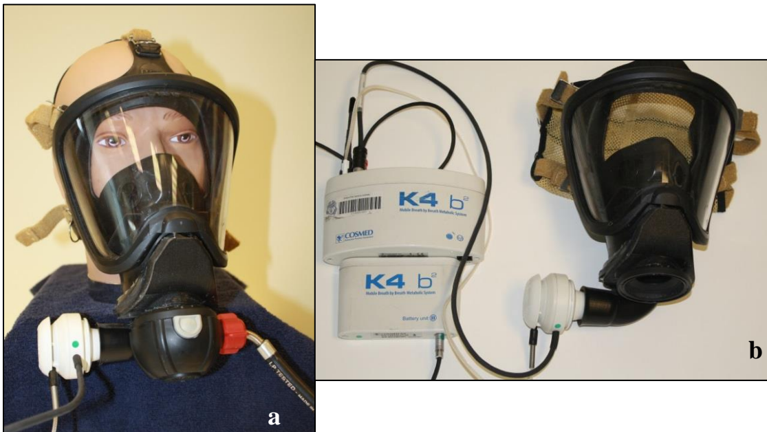
Figure 5. a) Complete modified SCBA facepiece assembly with Cosmed K4b 2 and SCBA regulator connected. b) Modified SCBA facepiece with Cosmed K4b 2 system.
