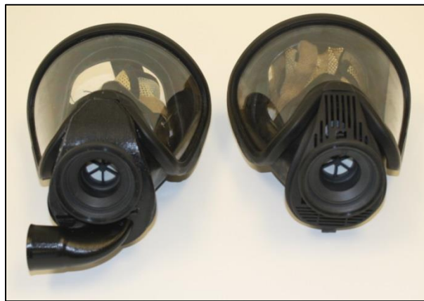
Figure 3. Modified facepiece (left) in comparison to the standard configuration (right).
