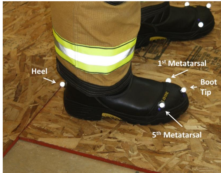
Figure 19. Passive reflective marker locations on the heel, first metatarsal, fifth metatarsal and tip of the boot.
