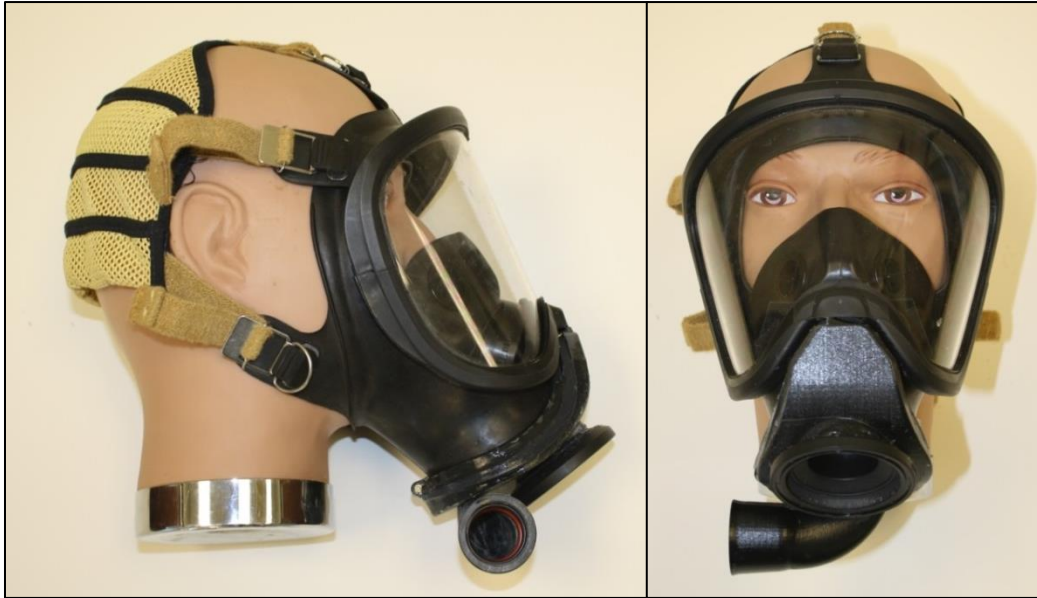
Figure 4. Front and side views of the MSA Firehawk M7 SCBA facepiece with modified component housing that accommodated the Cosmed turbine and gas sampling assembly via the calibration adapter.
