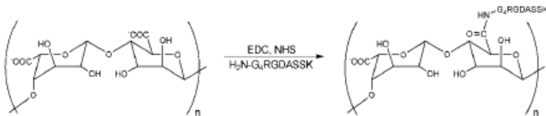
Figure 22 Conjugation of Arg-Gly-Asp (RGD) with alginate for enhanced cell adhesion in the microporous scaffold
