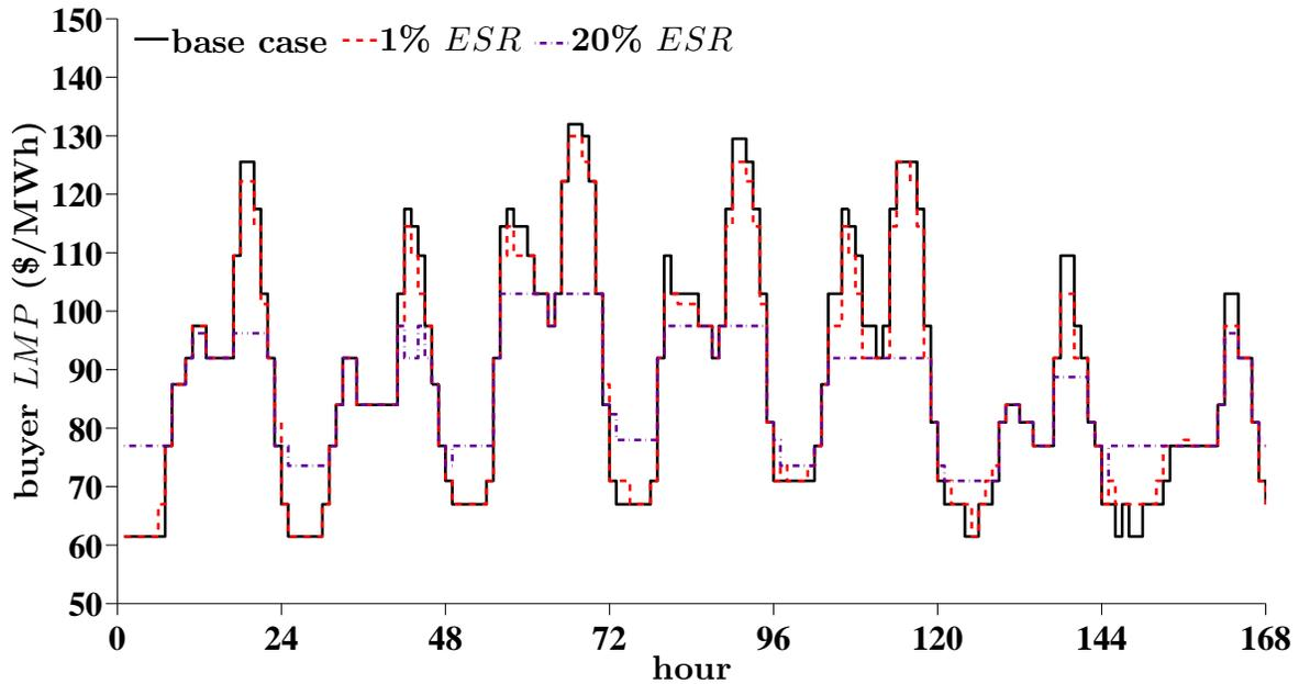
Figure 4.7: The hourly *LMPs* at bus 59 for the week of Dec. 13–19, 2010, on the  $MTS_{118}$
