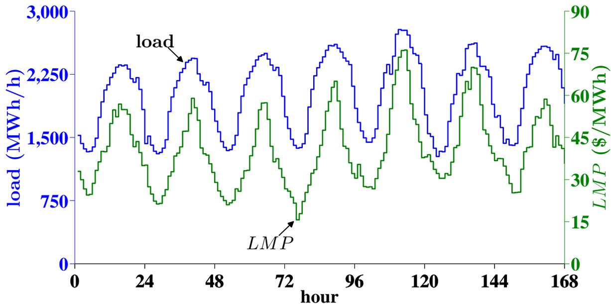
Figure 1.2: The hourly loads and the hourly  $LMP$ s for a load zone in *ISO-NE* for the week of July 12–18, 2010
