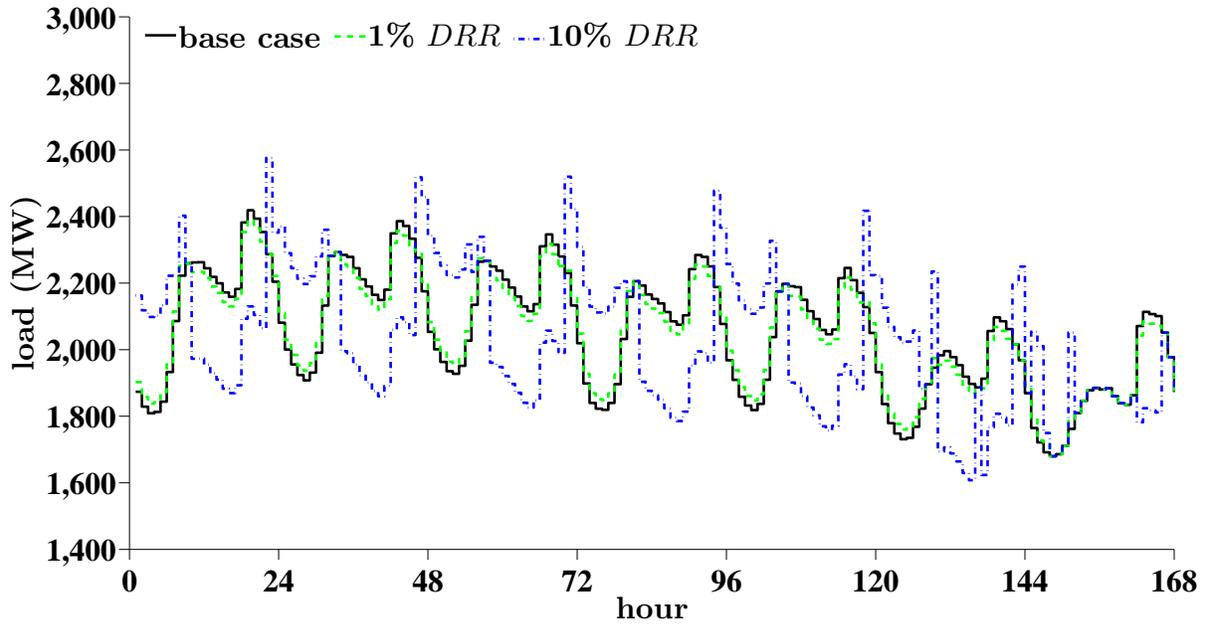
Figure 4.17: The hourly loads at bus 12 for the week of Dec. 13–19, 2010, on the  $MTS_{57}$
