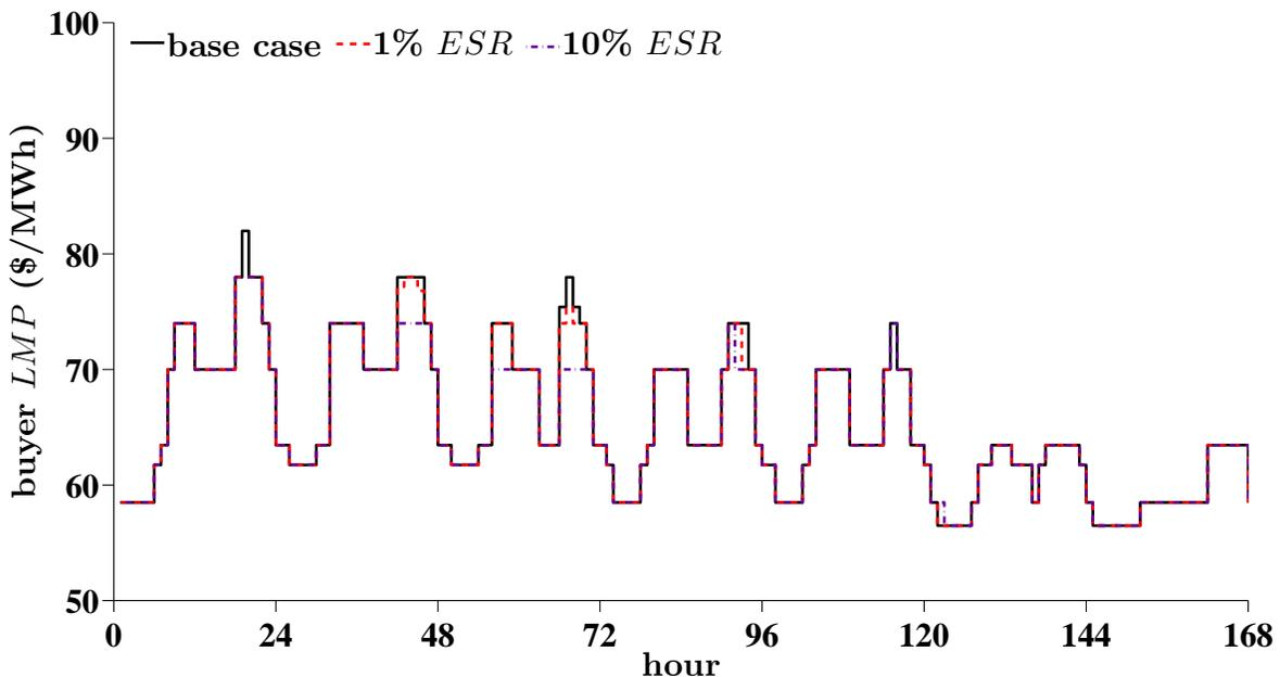
Figure 4.4: The hourly *LMPs* at bus 12 for the week of Dec. 13–19, 2010, on the  $MTS_{57}$
