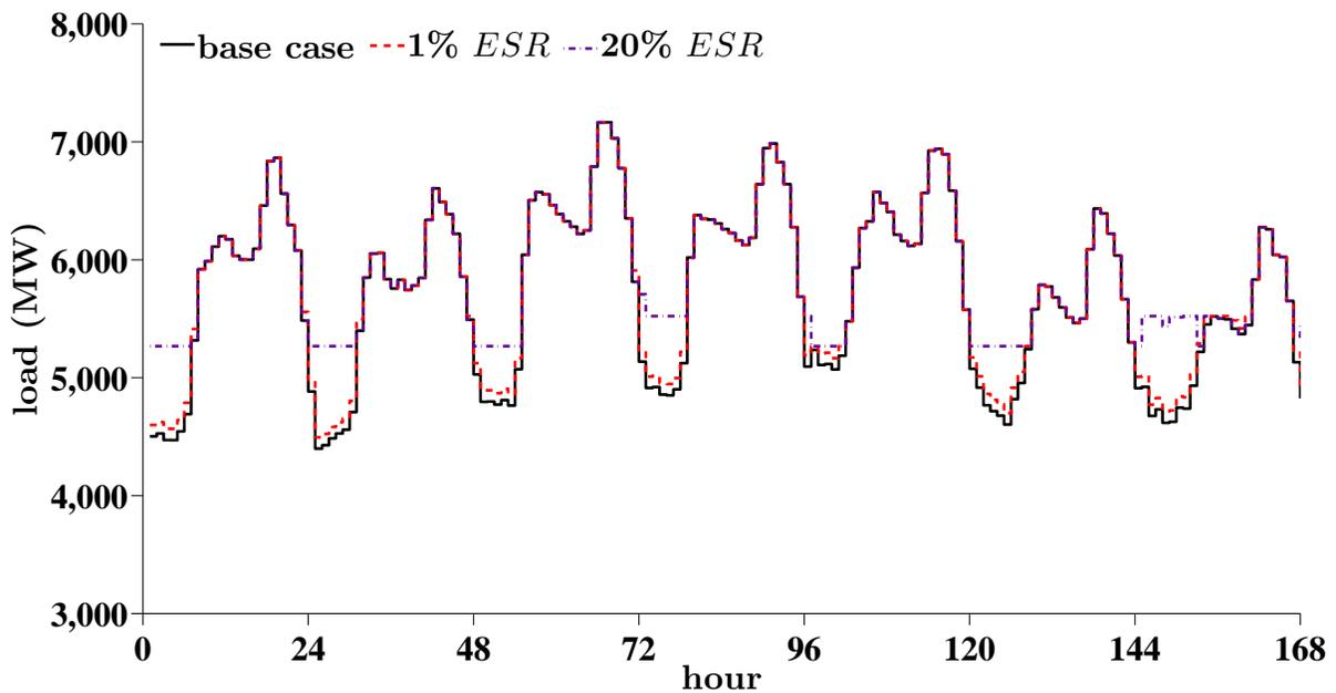
Figure 4.8: The hourly loads at bus 59 for the week of Dec. 13–19, 2010, on the  $MTS_{118}$
