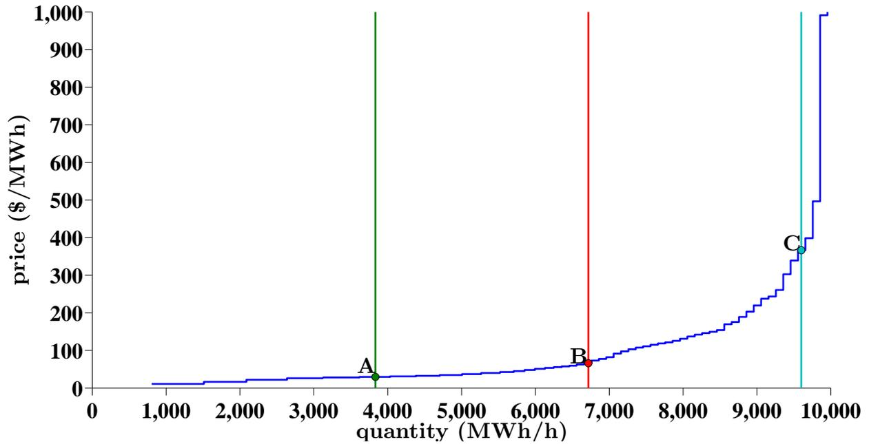
Figure 1.1: An *ISO-NE* offer curve for July 2010 with three load levels
