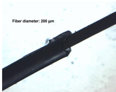
Figure 5.15 Optical microscope image of cross-linked poly(ECMS- co -DMS) coating on sacrificial PLA fiber.
