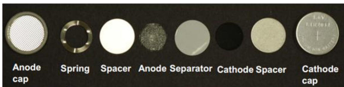
Figure 6.17 Assembling sequence of a lithium-ion coin cell battery. (Image courtesy of Marta Baginska)
