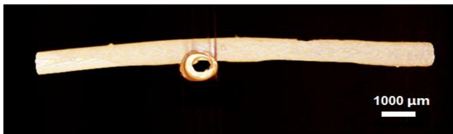
Figure 5.19 MicroCT image of two perpendicular, independent channels resulted from removing coated sacrificial PLA fibers.
