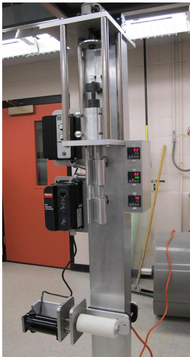
Figure 3.5 Photograph of the solution spinning setup. The PLA solution (dispersed with catalysts) is placed in the heated chamber. Using a motor-driven extruder, the PLA solution is extruded through the nozzle and excess solvent is evaporated as the extruded fiber passes through additional heating chambers. Extruded fiber is collected on a Teflon winder and dried.
