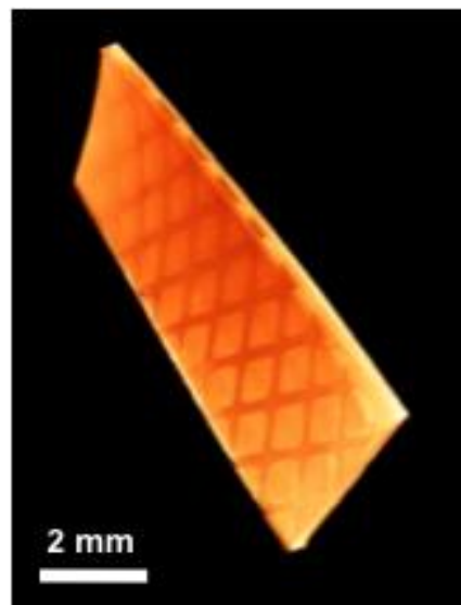
Figure 4.15 MicroCT Image showing the empty two-dimensional microchannels (diamond geometry) inside Ecoflex after VaSC process.
