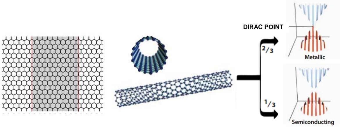
Figure 1.5 Diagram illustrating how the CNT can be considered a rolled up slice of graphene. Depending on the slice, the Dirac point can be included, yielding a metallic nanotube; otherwise, the nanotube is semiconducting [28].
