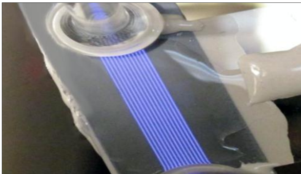
Figure 9. Photograph in plan view, showing the operation of a hybrid, 12 channel microplasma reactor operating in 1 atm of air.
