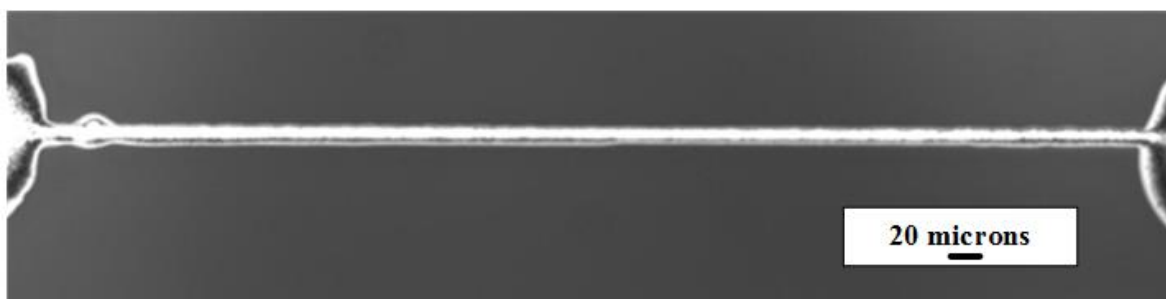
Figure 2.10 Optical microscope image of 20-pass AgDDB line (50% w/v Ag) printed with 5 \mu\text{m} nozzle after annealing.
