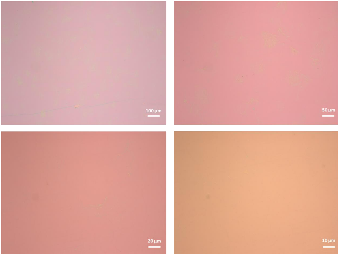
Figure 2.3 Optical microscope images of graphene synthesized on Cu foil and transferred on a clean 285nm thick SiO 2 /Si substrate with different magnifications.
