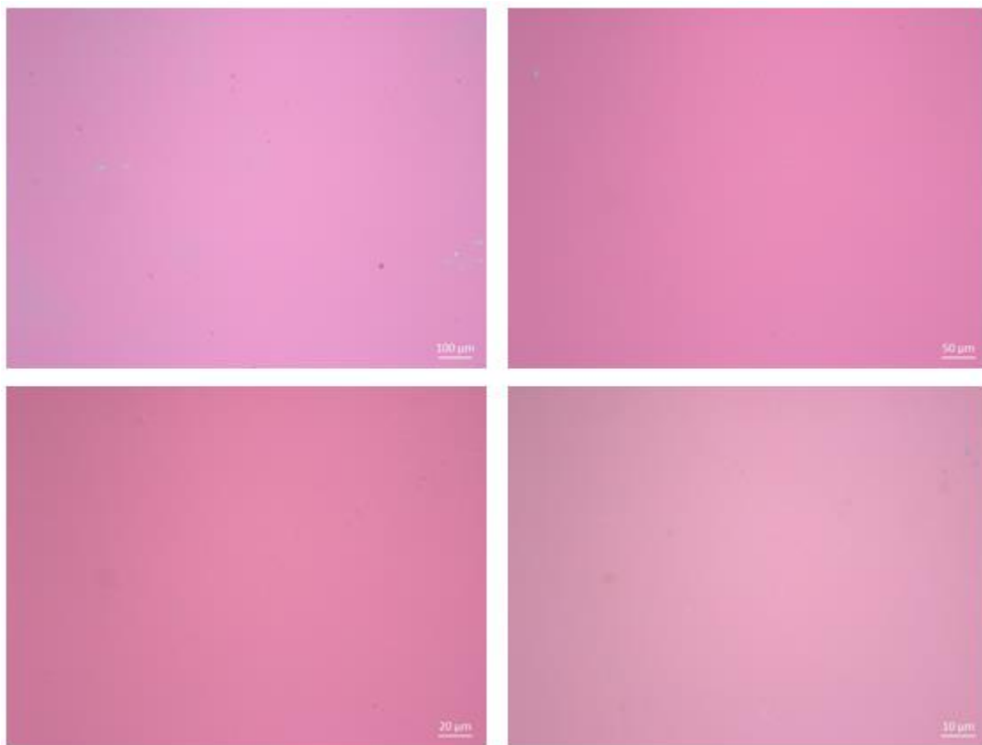
Figure 2.6 Optical microscope images of graphene synthesized on Cu film and transferred on a clean 285nm thick SiO 2 /Si substrate with different magnifications.
