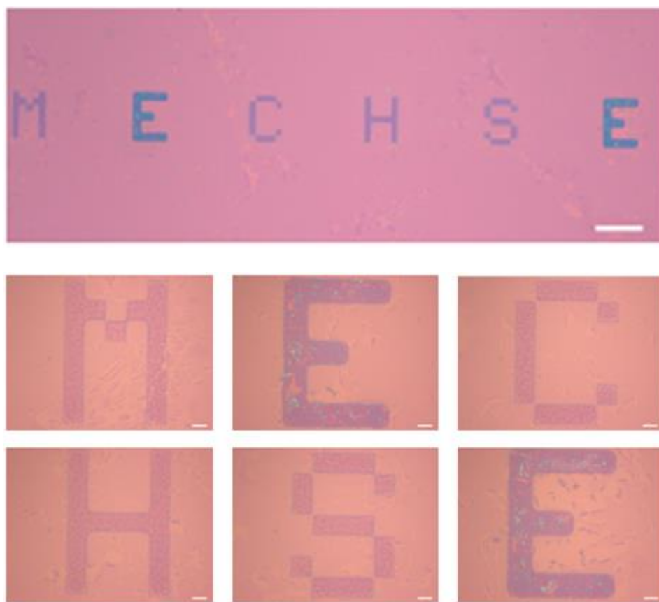
Figure 3.2. Synthetic control of graphene layers. Optical microscope images of graphene with different number of layers. Consonants are composed of thinner graphite and vowels are composed of thicker graphite. Background is composed of bi- to tri-layer garphene on a 285 nm thick SiO 2 /Si substate. Scale bars, 100 \mu m (top) and 10 \mu m (bottom).
