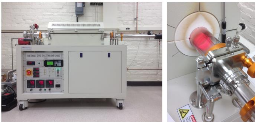
Figure 2.1 Actual LPCVD system for graphene and graphite synthesis: entire system (left), load lock (right).
