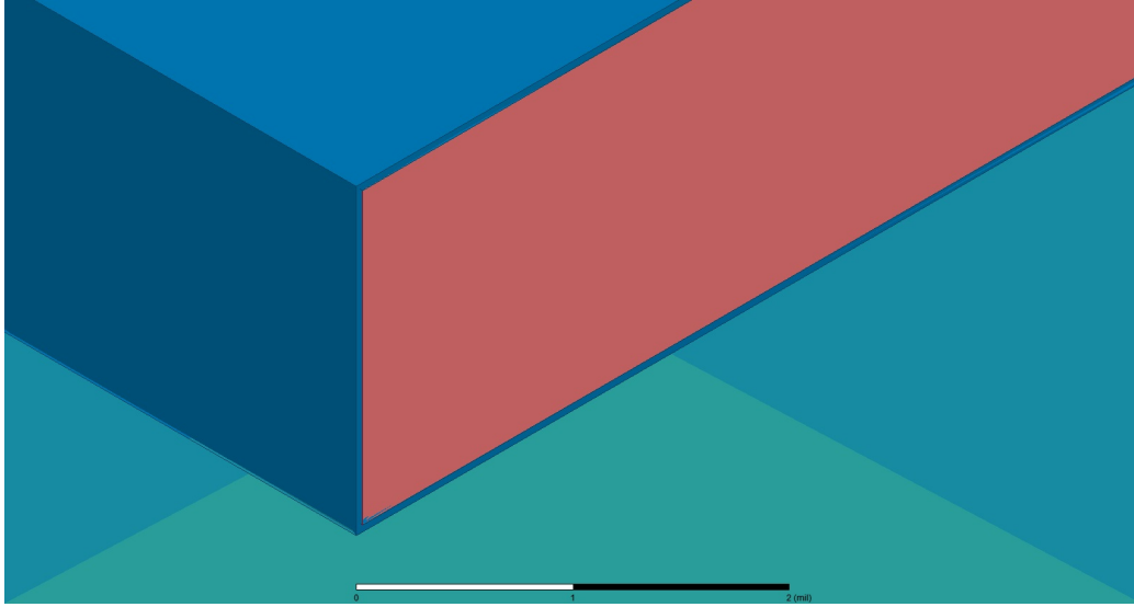
Figure 5.7: Close-up view of compound conductor structure in 3-D model of microwave filter in HFSS®
