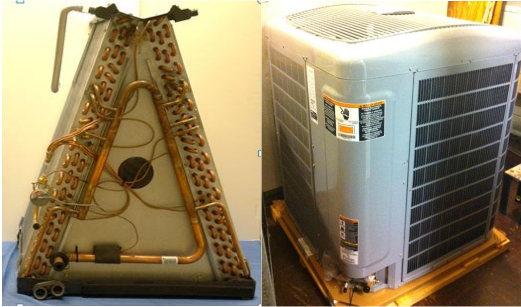
Figure 2.2: Pictures of indoor and outdoor heat exchangers (from left to right: indoor A-coil, outdoor coil)
