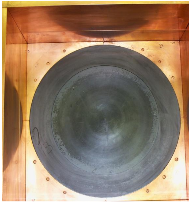
Figure 3.3: Zeus experiment fuel cavity looking down at the diaphragm from the top.
