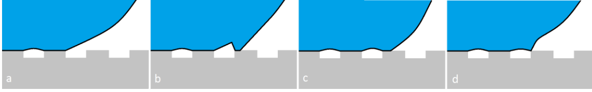
Figure 1.7: schematic showing the pinning criterion. (a) Configuration before pinning. (b) The facet closest to an unattached pillar is pinned. (c) The pinning is stable if the pinned facet does not collapse when evolved. (d) If the pinned facet destabilizes (in this case collapses into a corner), then the attached pillar fails the criterion. The critical pinning distance is determined as the maximum facet-pillar distance beyond which a pinned facet never stabilizes.
