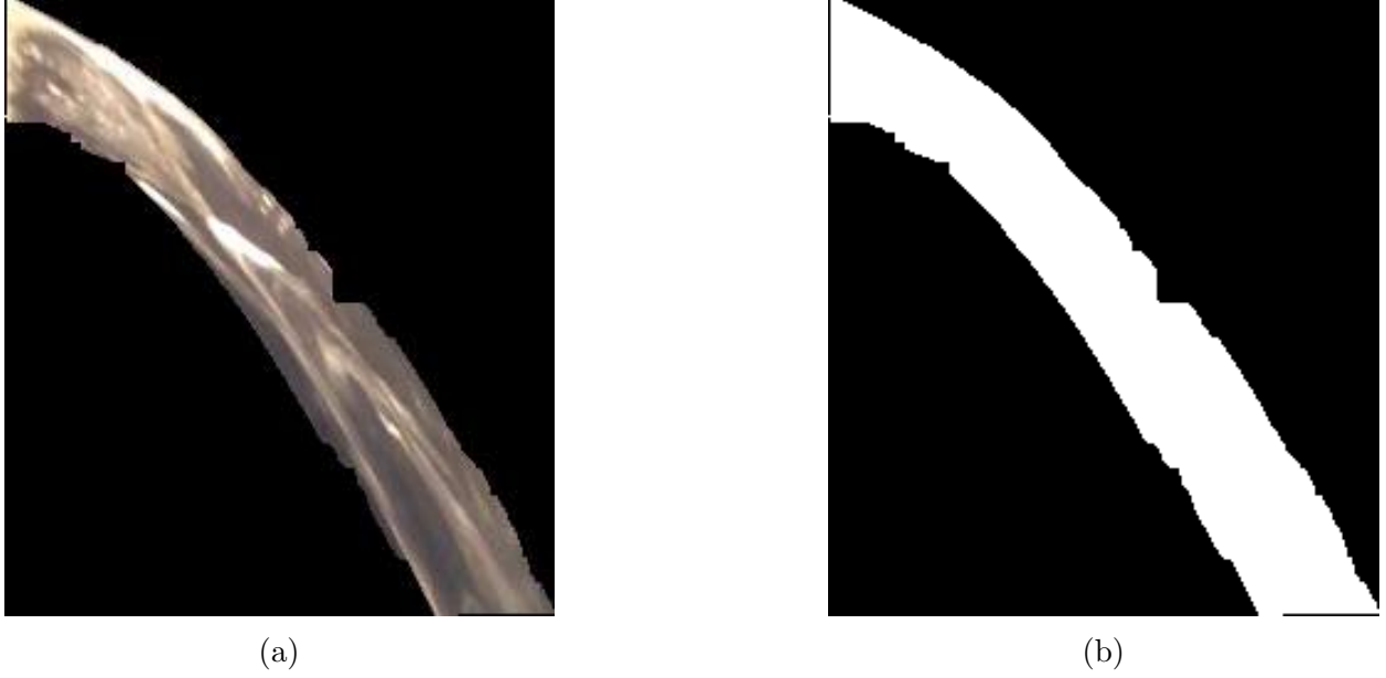
Figure 3.14: CSO detection sample frames. (a) Source image. (b) Detected binary image.
