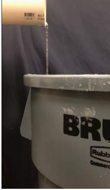
Figure 3.3: Demonstration of definition of overflow ends. Water flows out of the pipe and goes straightly down.
