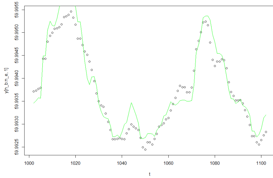
Figure 5.5: Frequency data re-creation (line indicates re-created data, points indicate simulated missing data) with 0.000327% average residual error
