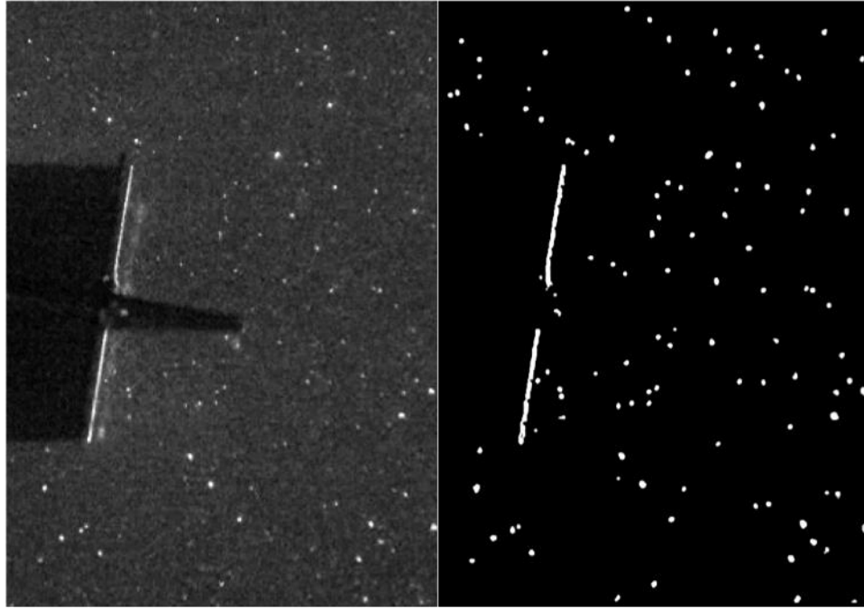
Figure 9: Typical image of miniature shear vane gray scale (left) and after frame exporting (right).
