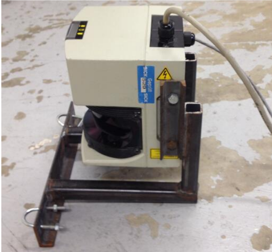
Figure 3.11 Modifications to the LIDAR unit
