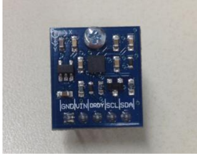
Figure 3.7 PARALLAX three axis HMC5883L electronic compass
