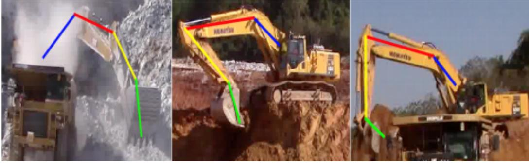
**Figure 4.1: Feature for training the CNN detection. We choose 5 important mechanical joints as the features to be fed into neural network model**
