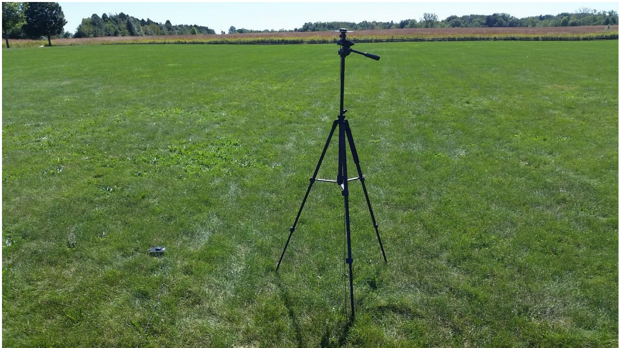
Figure 5- A Piksi basestation mounted on tripod in an open field. This was used as the primary GPS sensor for the ground control software. A tripod was required to minimize obstructions in order to enhance the reception quality of the GPS module, which improved the overall accuracy of the system. Stakes were used to secure the legs of the tripod into the ground in order to prevent wind gusts from knocking the tripod over.
