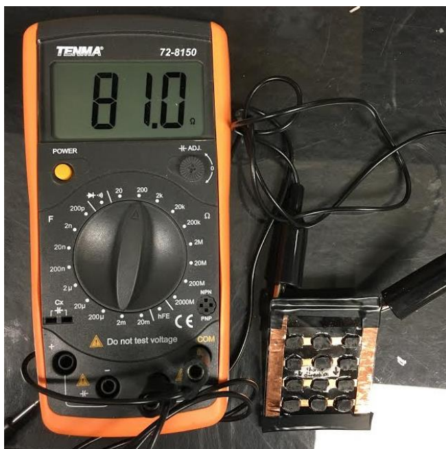
Figure 22. A second final device fabricated, with the resistance of the entire device shown using a multimeter. The final device has a resistance of 81 Ω.
