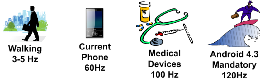
Figure 8.2: Guaranteed sampling frequency of Devices measuring gait. Human walking is usually in 3-5Hz which means to measure stepping a monitor of 10Hz sampling is enough.
