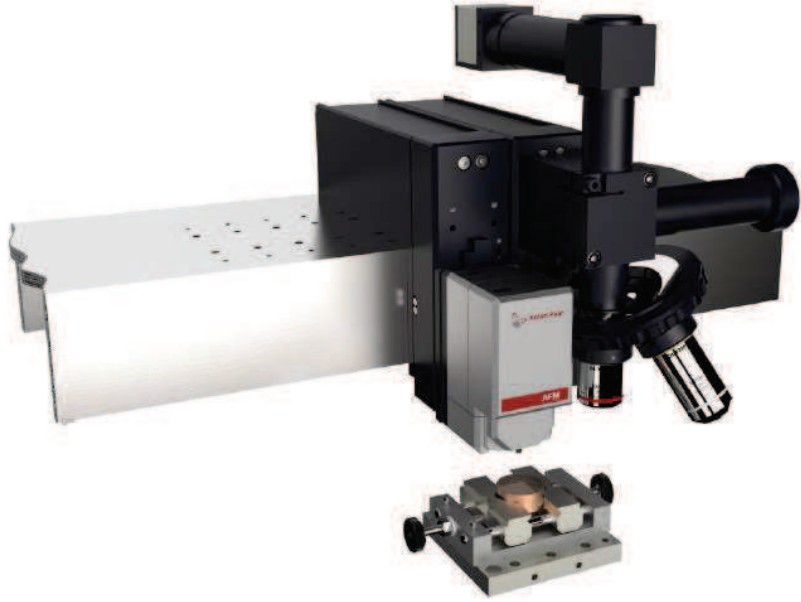
Figure 6.3: Micro Scratch Tester MST instrument (from Anton Paar Micro Scratch Tester MST Technical Features).
