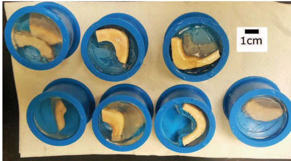
Figure 4.2: Cortical bone specimens embedded in PMMA after being ultrasonically cleaned.
