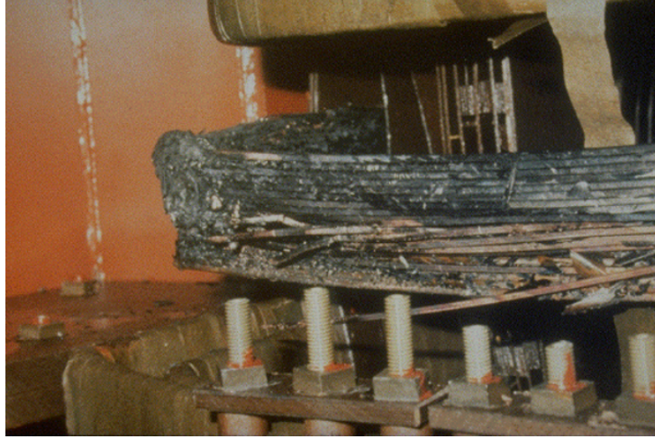
Figure 2.2: Transformer damage, adapted from [3]
