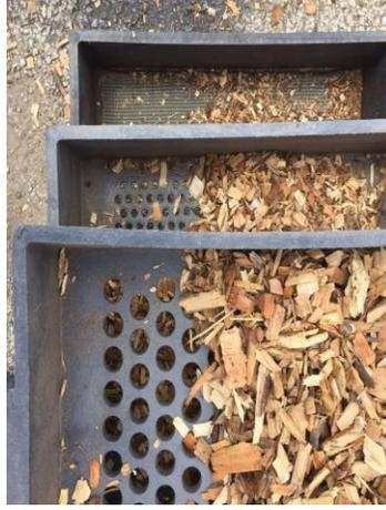
**Figure 3-4. Media separated into four particle size ranges.**
