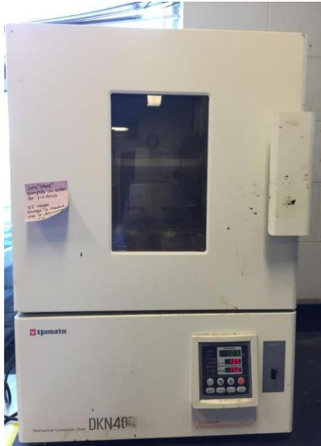
**Figure 3-8. Oven for drying biofilter media.**
