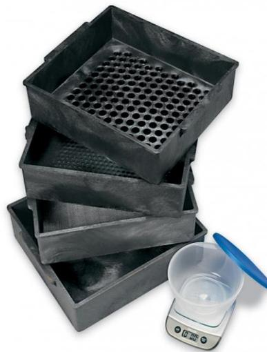
**Figure 3-3. Penn State Forage Particle Separator.**
