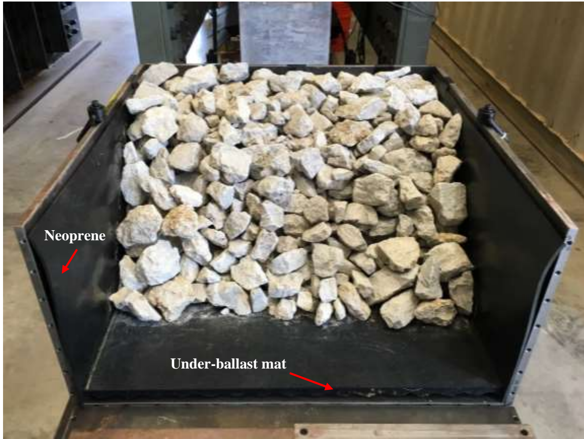
Figure 2.5 Profile view through open sidewall of the UIUC ballast box (demonstration only)
