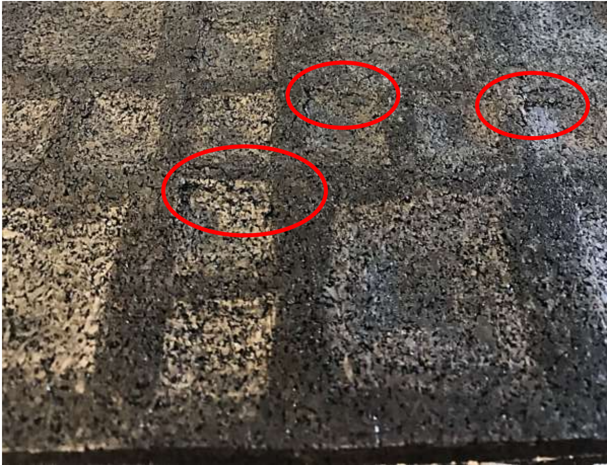
Figure 4.10 Example of cracks developed at edges of contact points for sample #3
