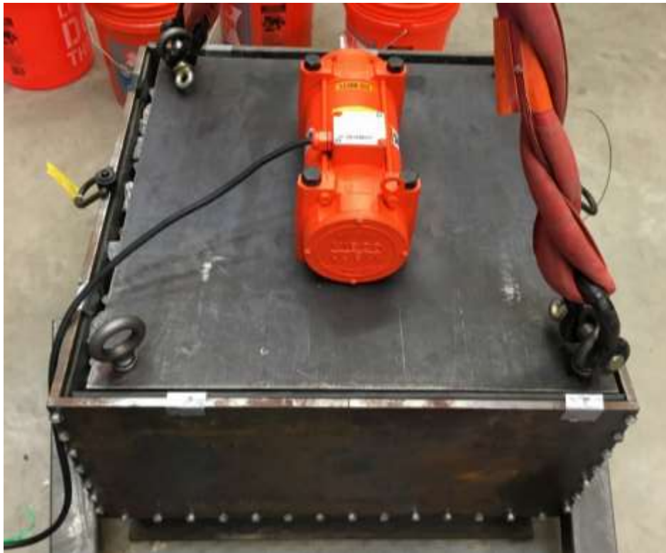
Figure 4.3 Compaction of ballast layer using vibratory plate
