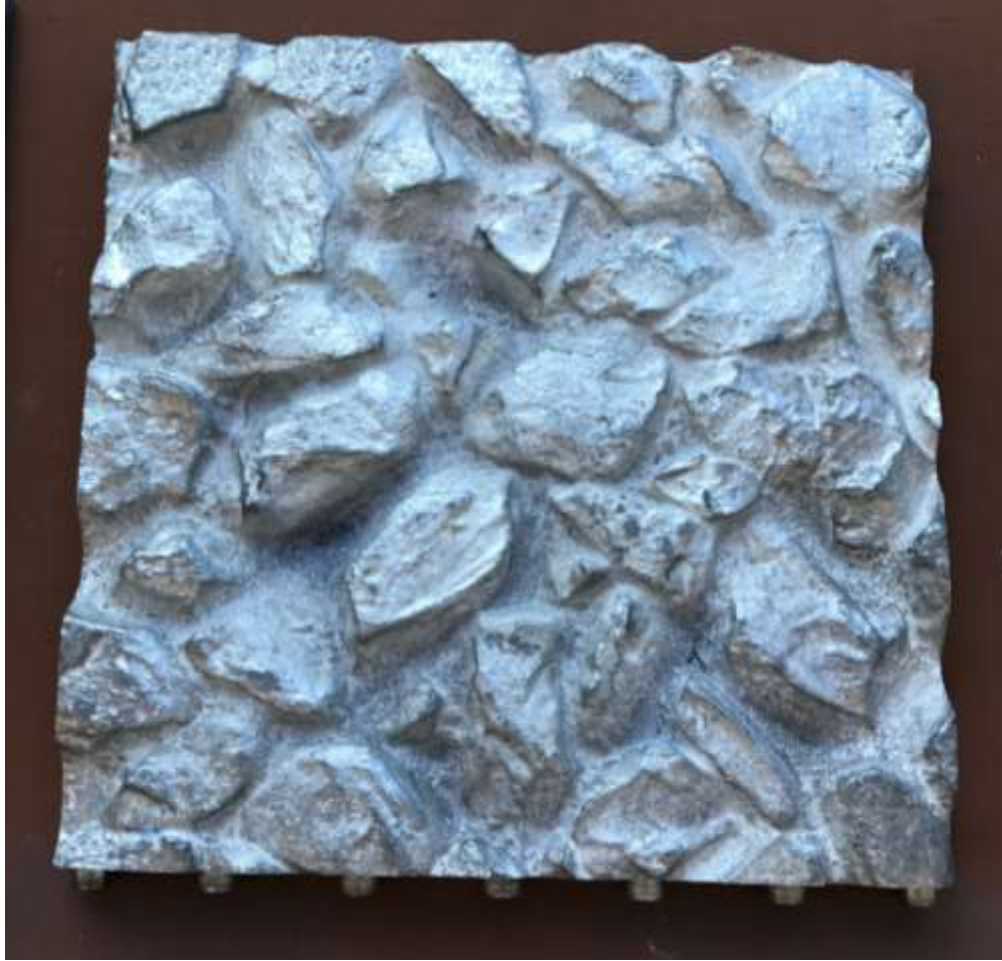
Figure 2.6 Plan view of a German DIN Ballast Plate at the Getzner Werkstoffe GmbH headquarters
