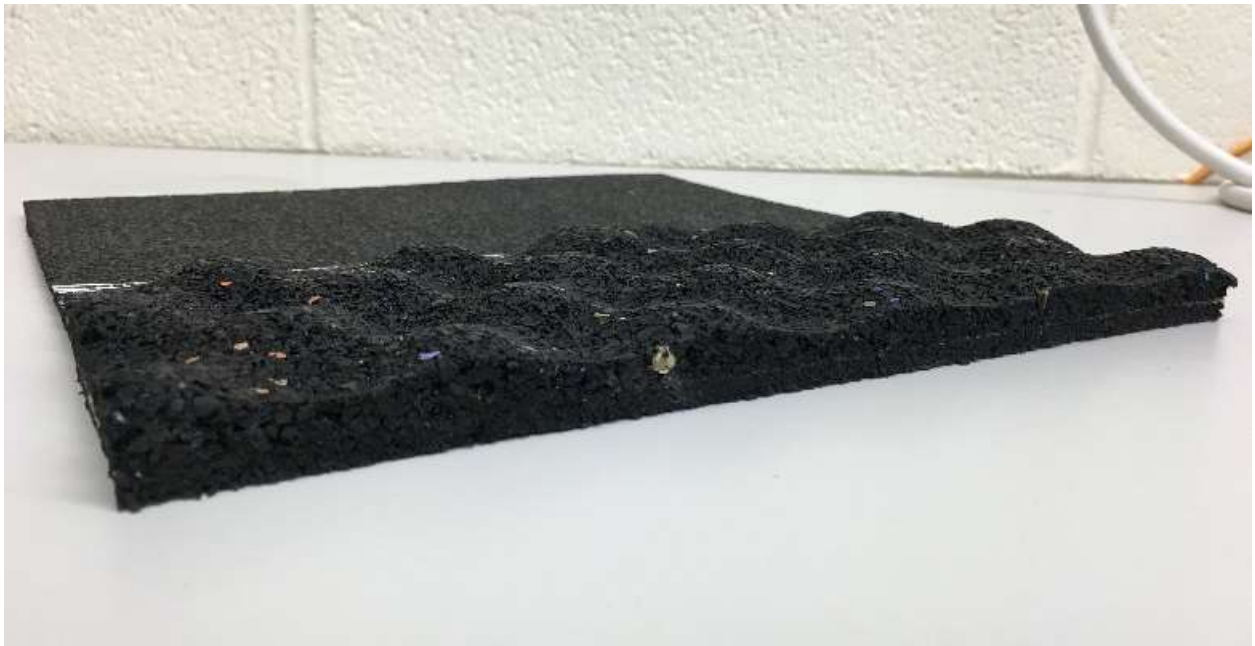
Figure 5.1 Type A UBM sample designed for freight loading
