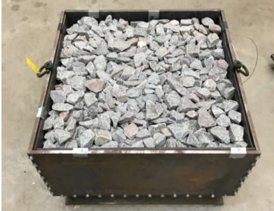
Figure 4.4 Finished compacted ballast layer in the UIUC ballast box
