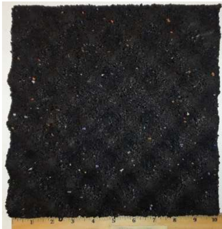
Figure 4.7 Type A UBM cut sample for GBP fatigue tests
