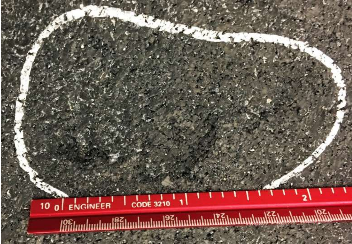
Figure 4.5 Superficial damage incurred to N.A. sample (ruler scale in inches)
