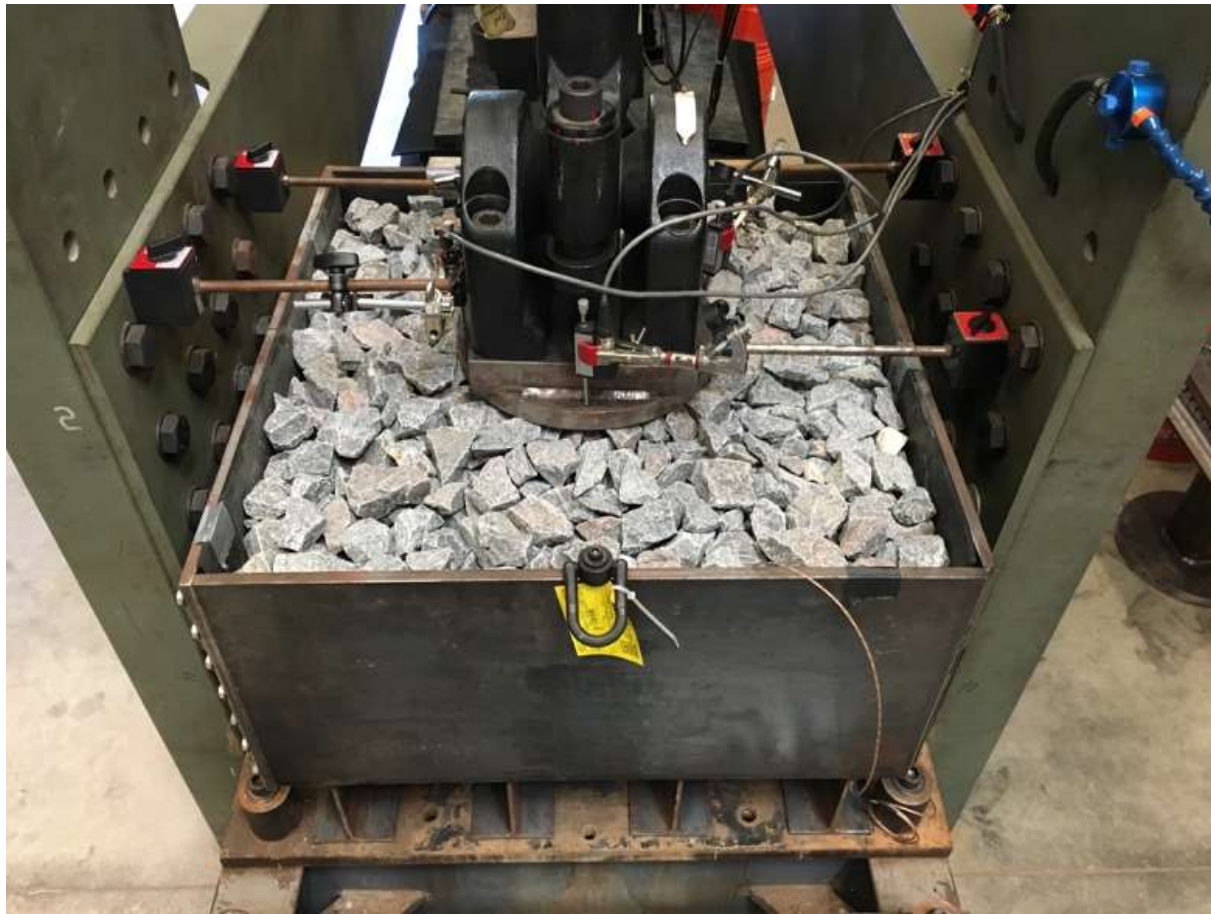
Figure 5.3 Constructed UIUC ballast box and loading plate setup with additional instrumentation
