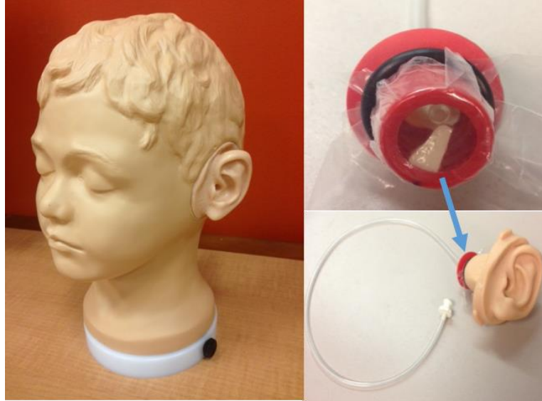
Figure 16. Ear model for phantom experiment. The middle ear cavity model can be filled with water or more viscous liquids. The TM is simulated by the thin plastic film (top-right).
