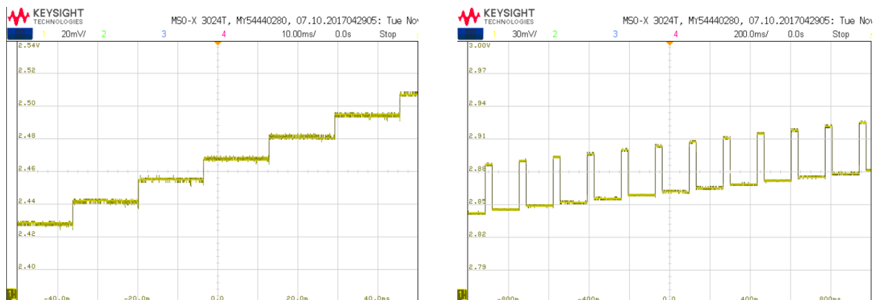
Figure 3.3 DAC output waveform CV (left), DPV (right).
