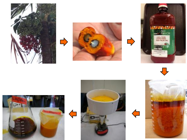
Figure. 2.5 Process of red palm oil fractionation. Red palm tree (top left), red palm nut (top center), commercial red palm oil (top right), Separation of different fats (bottom right), palm stearin (bottom center), and palm olein (bottom left; left) and palm stearin (bottom left; right). (Adapted from Garrow, 2015)
