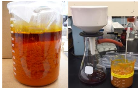
Figure. 2.4 Palm oil fractionation, crystallization process (left) and filtration (right).
